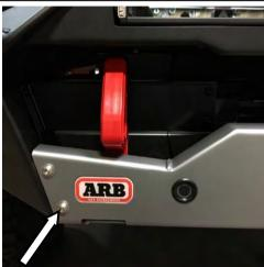
37. Place centre pan on vehicle and loosely fasten in place with 4x M8x20 stainless button head screws, stainless washers, and nuts.
