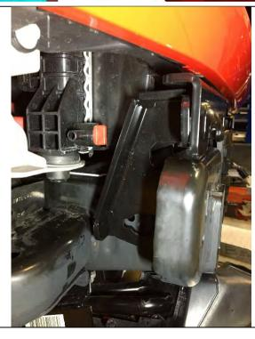
18. Using the same plastic nut that came off with the nut plates, secure the outer reinforcements on each side of the frame.
