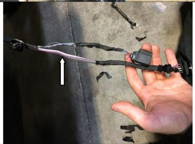
12. Using a razor, carefully strip back the loom to allow for more movement in the harness. Tape the exposed wires back up with black electrical tape.
