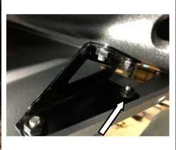
38. Using 4x stainless M6x16 button head screws, stainless washers, and nuts, fasten lower area of the centre pan to the mount brackets.
