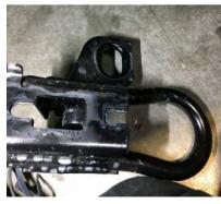
9. Remove bolts holding on factory tie down points and set aside. If these have the integrated intercooler mounts, they will be re-used.
