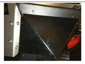
40. Slide these into place and attach with 3x black M6x16 bolts and black washers as well as 2x stainless M6x16 button head screws and stainless washers per side.
