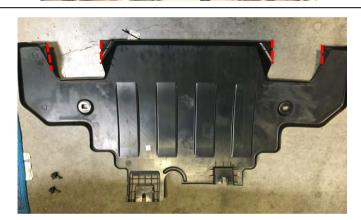
43. If your vehicle has a plastic stone guard with OE tow points, the area surrounding the tow points needs to be trimmed out as shown using an oscilatting multitool or jig saw.
