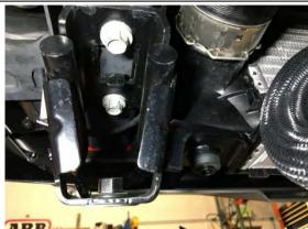
41. If vehicle came with front factory tie down points that incorporate the intercooler mounts, fit them back up now.
