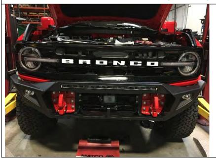
29. Place recovery points into bumper and then with the aid of another person or a lift table, carefully lift the bumper up to the vehicle. Using M12x50 bolts, washers (both sides of nut and bolt), and flange nuts, bolt the bumper loosely to the vehicle.
