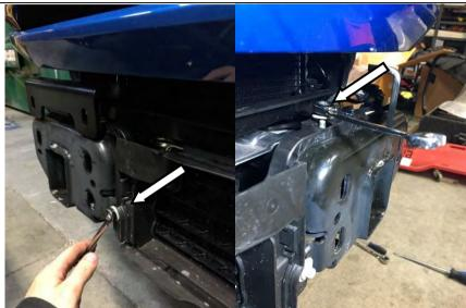
11. Remove the 4x bolts holding the ducting/shutters into the vehicle. Remove the connector and clips to get the harness off the shutters.
