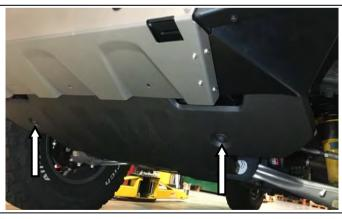
44. Refit the OE stone guard using the factory bolts as shown.
