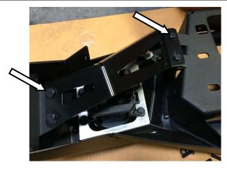
22. Using 4x M8x25 bolts, washers and flange nuts, bolt the reinforcement brackets to the bumper as shown.
