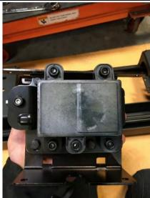
23. Assemble the radar (if equipped) as shown with 3x M6x16 bolts, washers, and flange nuts.
