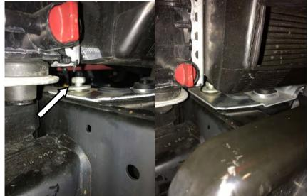
14. Loosen the top intercooler mount plate. This is a tight area to get tools into. Remove the bolt on each side and set aside for chassis bracket fitment.
