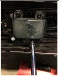
10. Remove factory radar cover and radar (if optioned) by removing the 3x screws under the cover. Set these both aside as they will be re-used.
