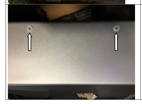
34. Install 2x plastic gromets into the centre pan as shown for the licence plate (if required).
