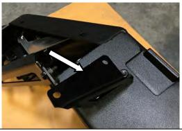
28. Using 3x M12x70 bolts, washers, and flange nuts per side, assemble recovery points as shown.
