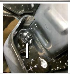
8. Remove factory nut plates by loosening plastic nut on back of the chassis end plate.
