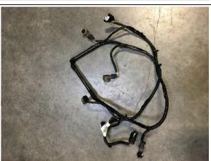
7. Remove the wiring harness for the parking sensors and fog lights and set aside for fitment into the ARB bar.
