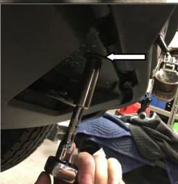
Remove 6x bolts holding the under tray on and retain for refitting the under panel later.
