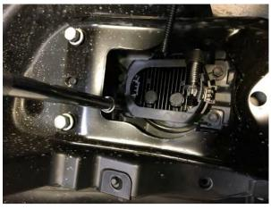
6. If fog lights are installed, remove these and set aside for later.
