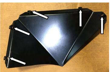
39. Using 5x M6 cage nuts per side, assemble wing under panels as shown.
